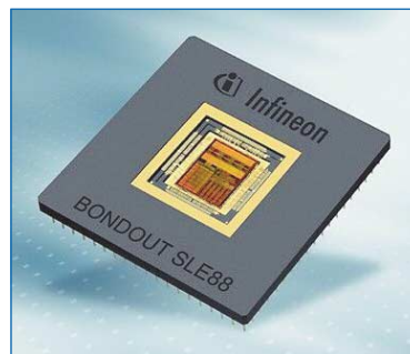
Bondout-Version des 32-bit Chipkartencontrollers SLE88CFX4002P.
